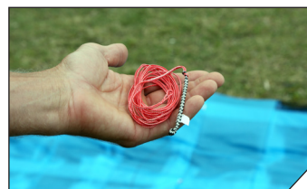
2 Unwind the LSL line (included in spares kit, labeled #5). Ensure there are no tangles or knots in the line.
