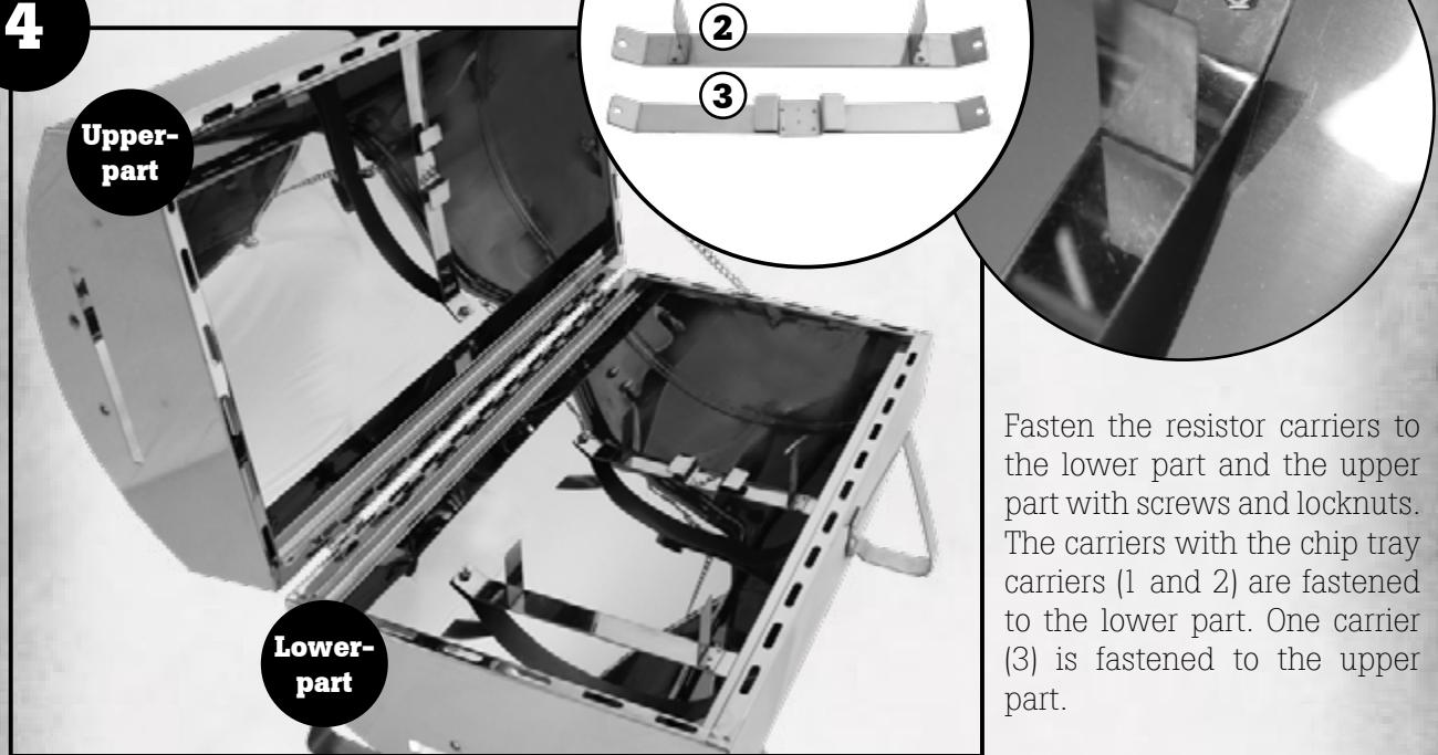
Fasten the resistor carriers to the lower part and the upper part with screws and locknuts. The carriers with the chip tray carriers (1 and 2) are fastened to the lower part. One carrier (3) is fastened to the upper part.
